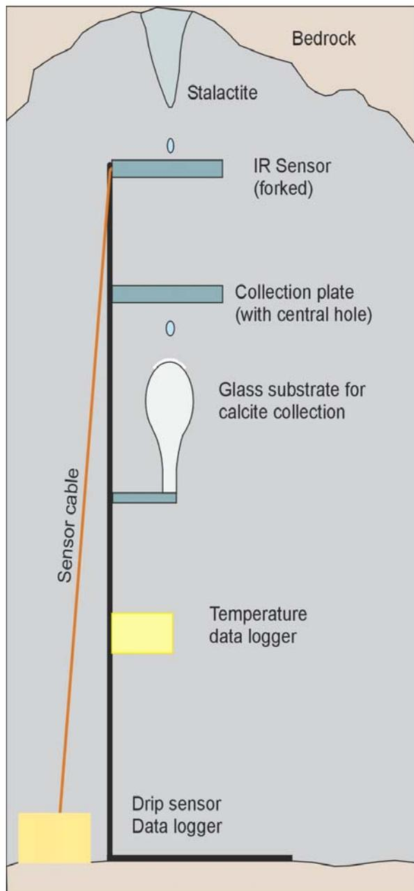
**Figure 3:** Schematic of discharge monitoring apparatus. Discharge recorded by the IR sensor was downloaded from the data logger ~ monthly intervals. Bottle for water collection for chemical analysis was placed on the collection plate. Calcite was precipitated onto the glass substrate and collected at intervals as determined by growth rate and frequency of visits.
