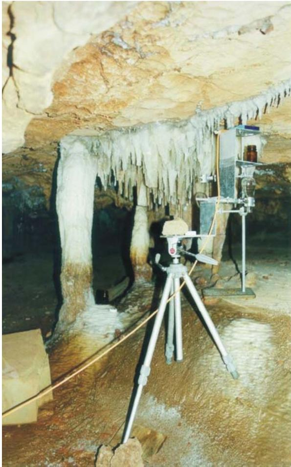
**Plate 3:** The automatic discharge monitoring apparatus set up in Wollondilly Cave at a bedrock thickness of 45 m. Photo: J. McDonald.
