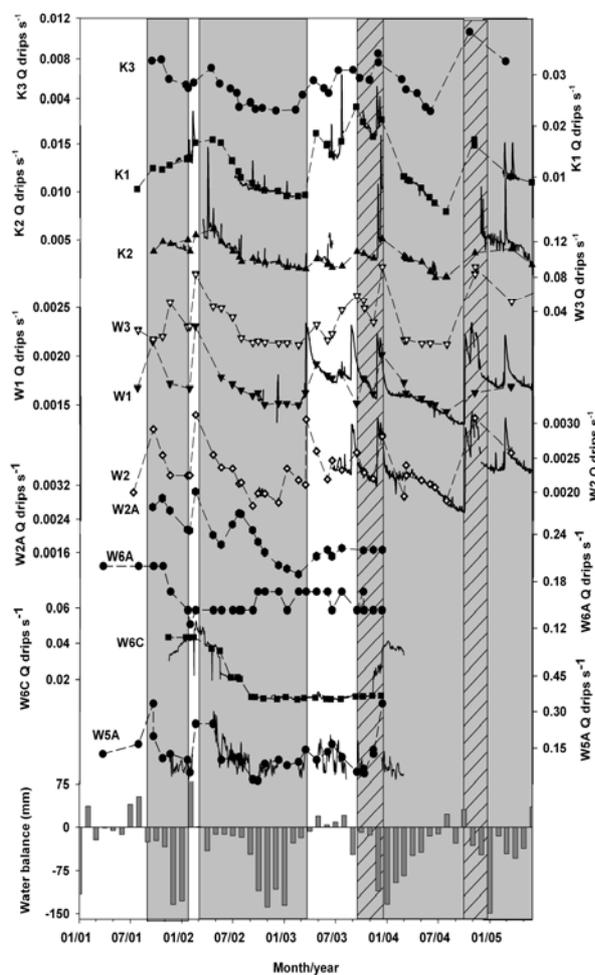
**Figure 4:** Discharge and site water balance profile for all sites in according to bedrock thickness. Symbols are manual readings and solid lines are automatic drip-sensor values. The grey shaded phases are water-deficit periods. The stippled areas are periods of transient water excess due to spring/summer storms, resulting in recharge to the shallow sites.
